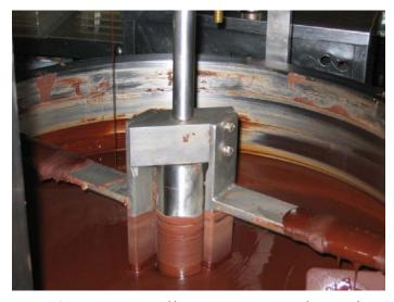
Temperers are tempering machines with computer controls that produce consistent tempered chocolate for large volumes. While a *Temper Meter* measures the temper of the chocolate, and ensures accuracy and consistency.
