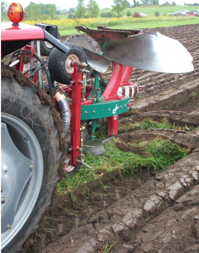
Source: Slide 60– Plowing 101 Back coulters should cut the last of the unplowed soil but not cut the Crown furrow.
