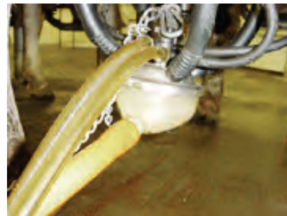
If milk letdown has been properly stimulated, then milk will start flowing freely in the claw shortly after applying the machine.
