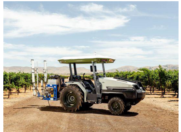
Monarch Electric Tractor, developed in California. This tractor is also designed to be autonomous.
