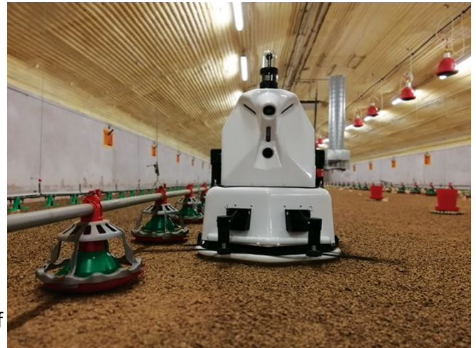
Octopus Poultry Safe autonomously sanitizes and decontaminates large buildings while collecting environmental data.
