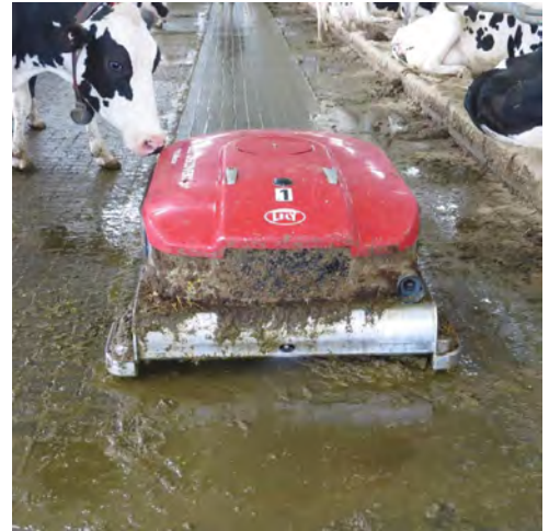
Lely Discovery 120 Collector working to vacuum up manure in a sand-bedded barn.
