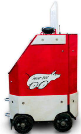
The Boar Bot robot helps the boar check for sows that are in heat.
