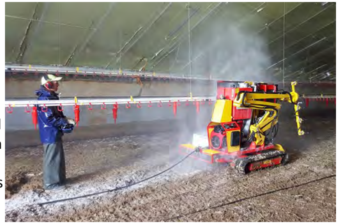
Lavicole high-pressure washing robot for poultry barns Image Credit: Rabaud
