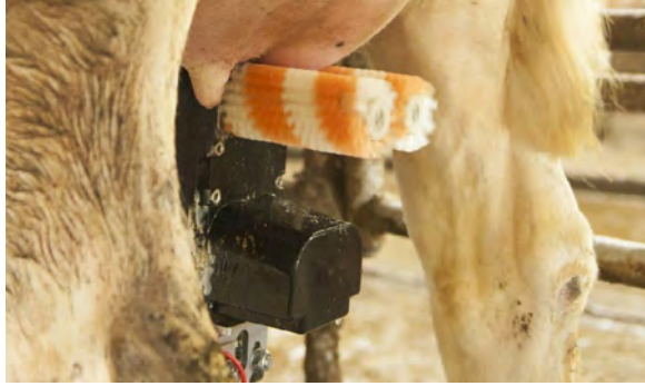
Robot brushing the teats to clean them and stimulate the cow to let her milk down
