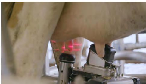
The laser on the robotic milker searches out the teat on the cow to find where to place the milk cup.
