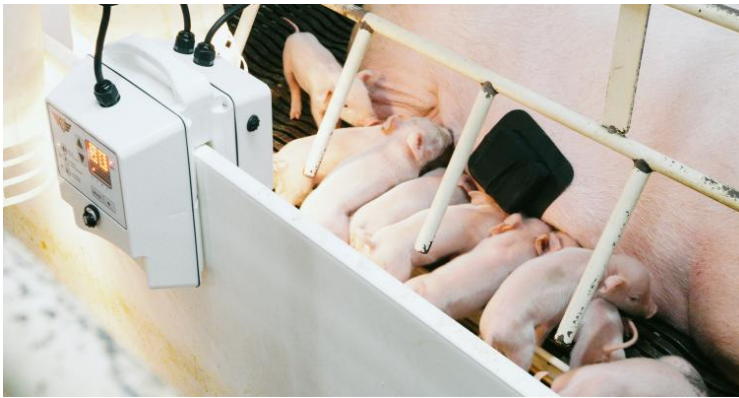
Protecting Pigs - a sow wears a SwineTech patch, which works with the device hanging on the farrowing stall. Designed to prevent baby pigs from being crushed to death, the system sends a vibration to the sow to move.
